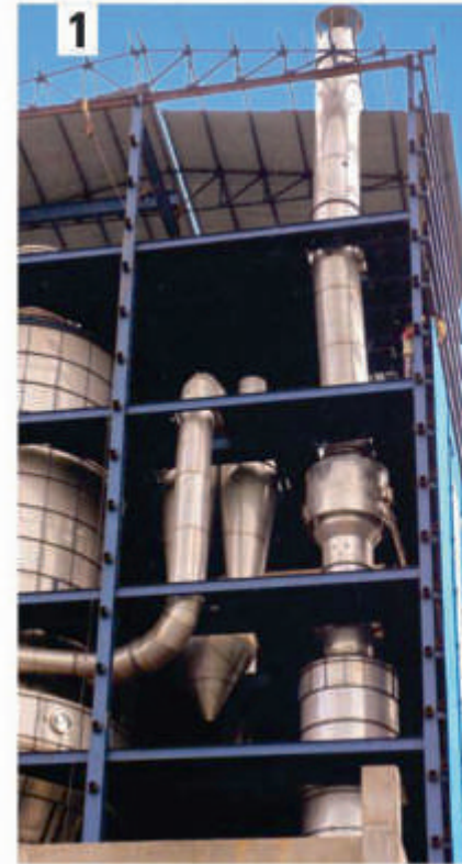
1) High Efficiency Twin Cyclones with Two Stage Ventury Scrubber having Swirler Flasher
